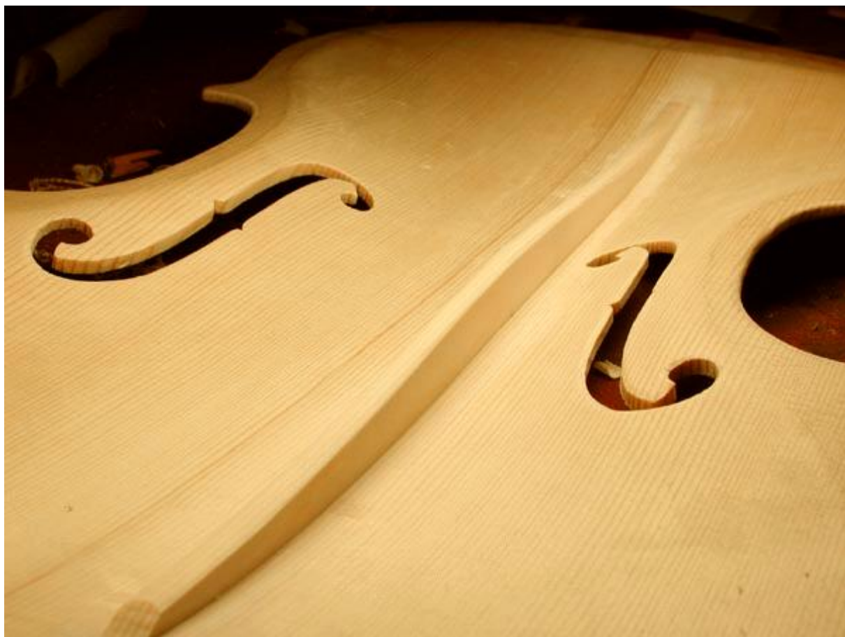
The belly from inside with f-holes cut and bassbar fitted.
