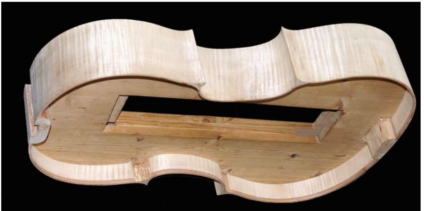
Cello ribs with linings
