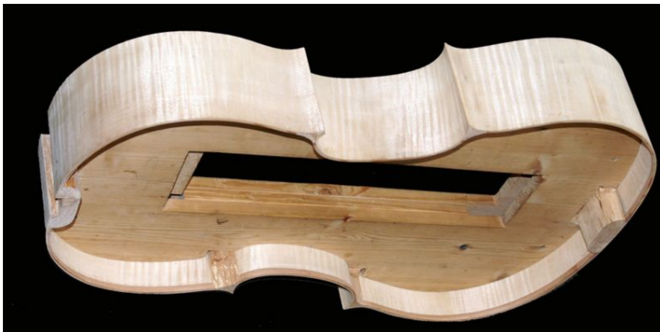
Cello ribs with linings
