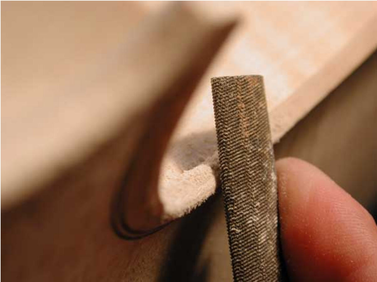
Chamfering the back edges
