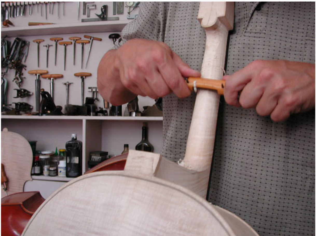
Blending the neck with an edge flayer.
