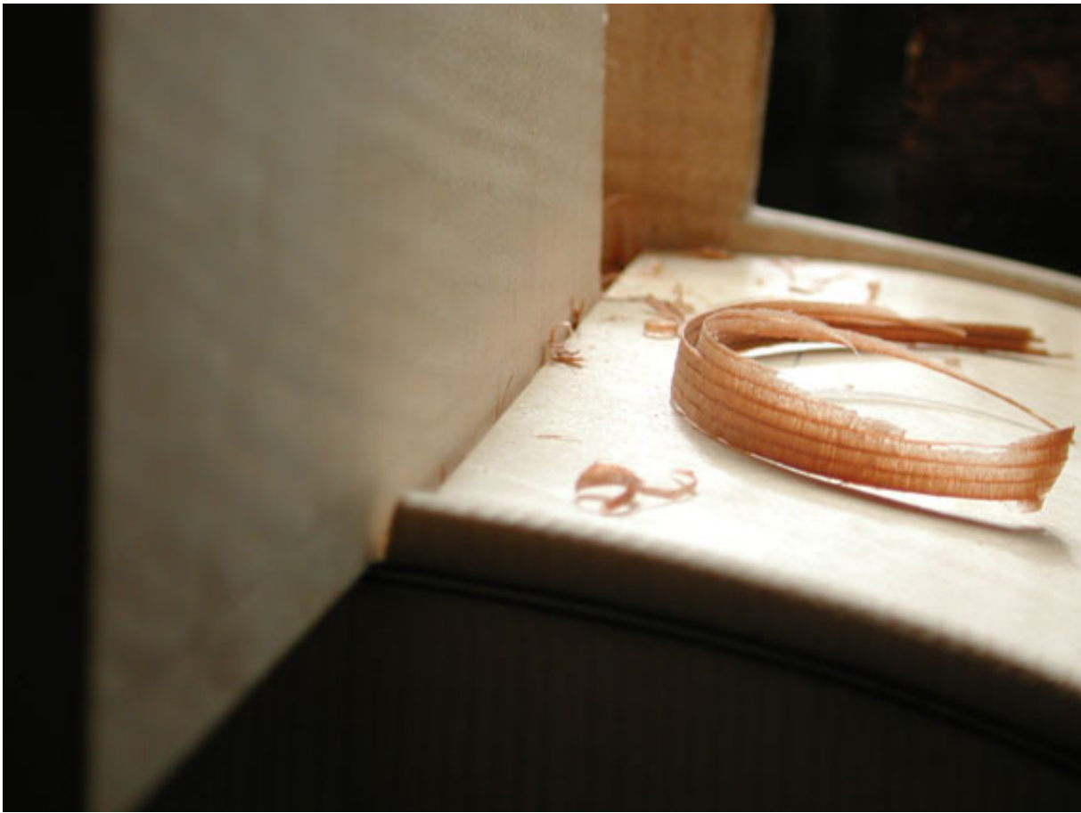
The base of the neck is slowly fitted into the cut-out.
