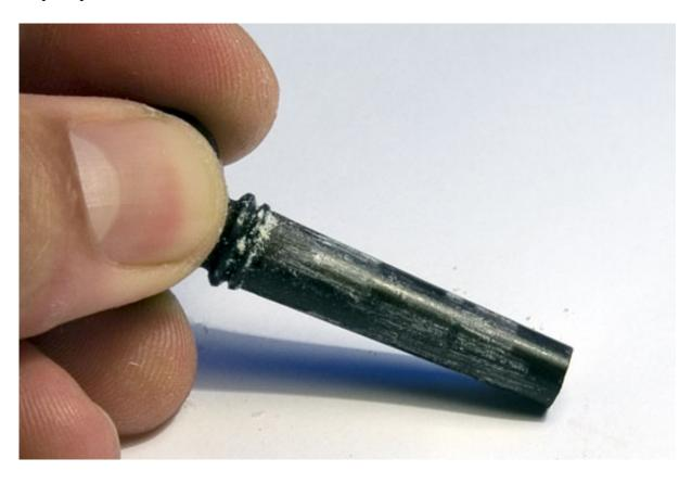
Clear to see: This peg does not sit properly and has to be refit. To be sure that the peg hole is round, it is carefully rethread with a so-called peg reamer:
