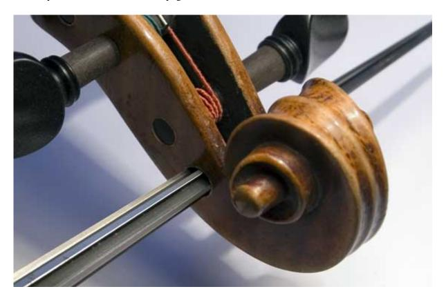
The next task consists of recutting the peg with a peg shaper. The peg shaper shown in the photo can be adjusted to any cone and peg diameter by means of a moveable carriage and allows for the finest reduction of wood shavings.
